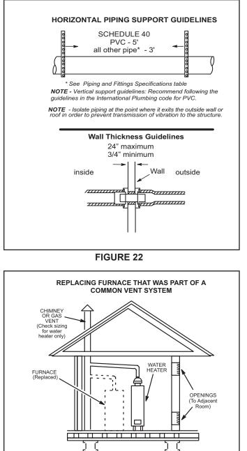
If replacing a furnace which was commonly vented with another gas appliance, the size of the existing vent pipe for that gas appliance must be checked. Without the heat of the original furnace flue products, the existing vent pipe is probably oversized for the single water heater or other appliance. The vent should be checked for proper draw with the remaining appliance.
