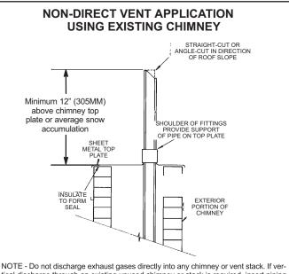
NO IE - Do not discharge exhaust gases directly into any chimney or vent stack. If vertical discharge through an existing unused chimney or stack is required, insert piping inside chimney until the pipe open end is above top of chimney and terminate as illustrated. In any exterior portion of chimney, the exhaust vent must be insulated.
