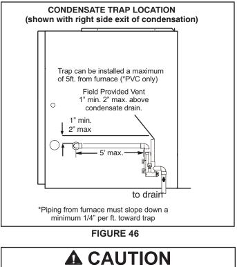
Do not use copper tubing or existing copper condensate lines for drain line.
