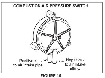
**NOTE** - The switch is factory set and is not field adjustable. It is a safety shut-down control in the furnace and must not be by-passed for any reason. If switch is closed or bypassed, the control will not initiate ignition at start up.
