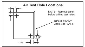
FIGURE 5. Air Test Hole Locations
