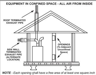
per 1,000 Btu ( $645mm^2$  per .29kW) per hour of the total input rating of all equipment in the enclosure, but not less than 100 square inches ( $64516mm.^{2}$ ).
