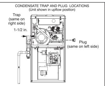
NOTE - In upflow applications where side return air filter is installed on same side as the condensate trap, filter rack must be installed beyond condensate trap or trap must be re-located to avoid interference.
