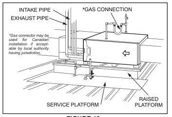
FIGURE 19 Return Air -- Horizontal Applications
