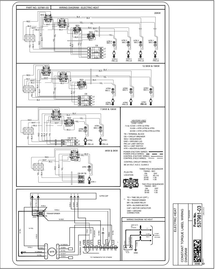
FIGURE 21. Unit Wiring Diagram – Electric Heat and Air Handler
