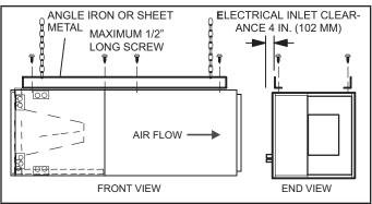
FIGURE 12. Suspend Horizontal Unit
