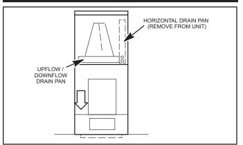
FIGURE 16. Downflow Discharge Position
