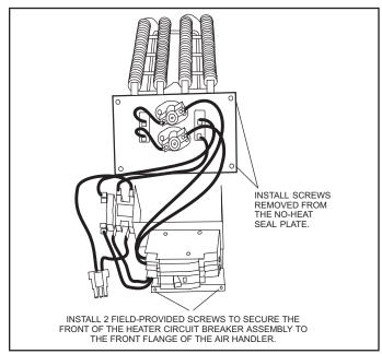
FIGURE 5. Installing the Heat Element Assembly
