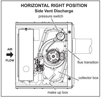
The SL280UHV series units are classified as fan-assisted Category I furnaces when vertically vented according to the latest edition of National Fuel Gas Code (NFPA 54 / ANSI Z223.1) in the USA. A fan-assisted Category I furnace is an appliance equipped with an integral mechanical means to either draw or force combustion products through the combustion chamber and/or heat exchanger. The SL280UHV is not approved for use with horizontal venting.
