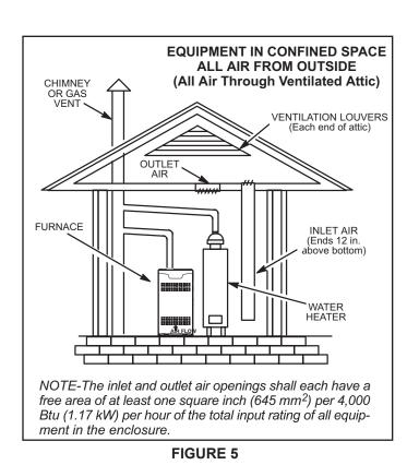
NOTE - Each air duct opening shall have a free area of at least one square inch (645 mm²) per 2,000 Btu (.59 kW) per hour of the total input rating of all equipment in the enclosure. If the equipment room is located against an outside wall and the air openings communicate directly with the outdoors, each opening shall have a free area of at least one square inch (645 mm²) per 4,000 Btu (1.17 kW) per hour of the total input rating of all other equipment in the enclosure.
