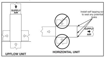
**NOTE -** Do not operate the furnace in the heating mode with an external static pressure that exceeds 0.8 inche w.c. Higher external static pressures may cause erratic limit operation.
