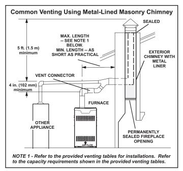
DO NOT insulate the space between the liner and the chimney wall with puffed mica or any other loose granular insulating material
