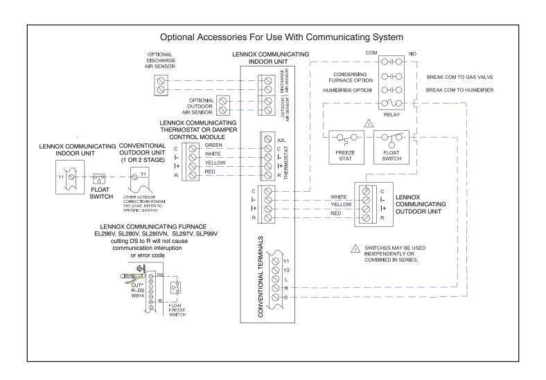
**TABLE 8**SL280 Field Wiring Applications With Conventional Thermostat
