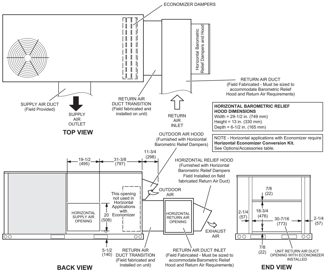
**NOTE** - Return Air Duct and Transition must be supported.
