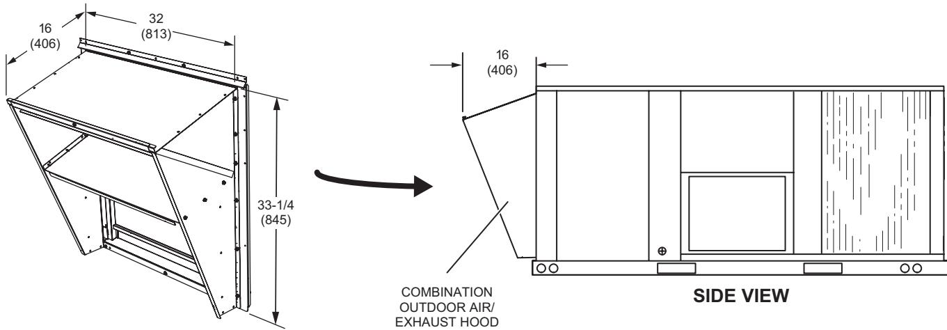
**OUTDOOR AIR DAMPER HOOD DETAIL (Downflow or Horizontal Applications)**
