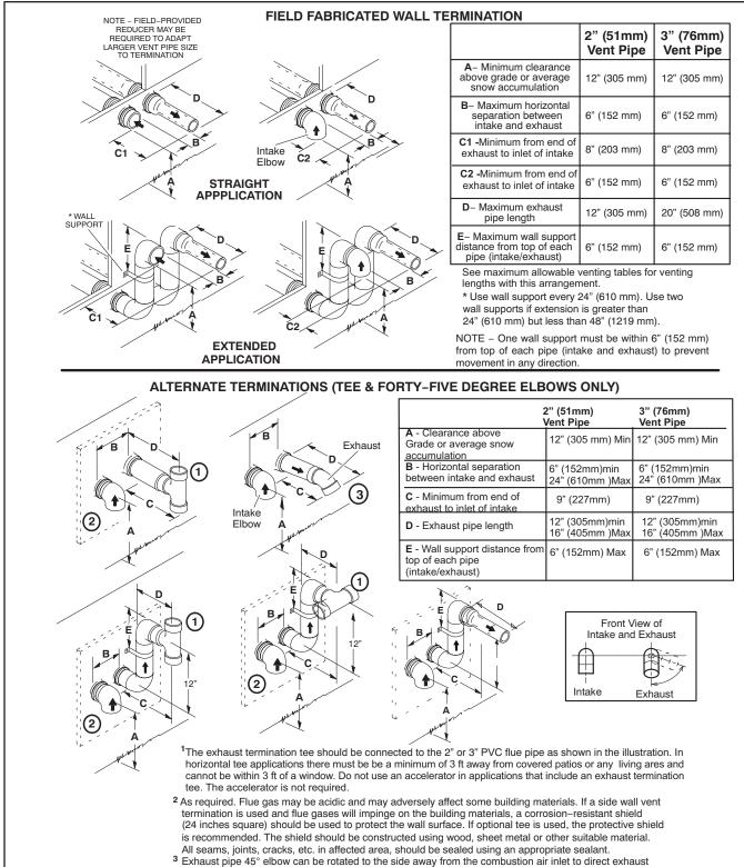
\* Exhaust pipe 45° elbow can be rotated to the side away from the combustion air inlet to direct exhaust away from adjacent property. The exhaust must never be directed toward the combustion air inlet.
