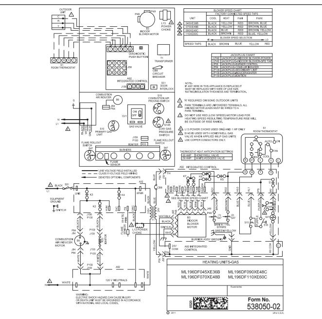
1 - Line voltage is applied to L1 and N. the T1 low voltage transformer is energized, and line voltage is applied to B3 indoor blower.
