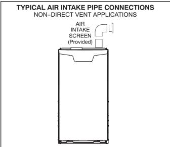
**NOTE** - Air intake screen and elbow may be rotated, so that screen may be positioned to face forward or to either side.
