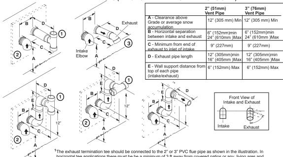
horizontal tee applications there must be be a minimum of 3 ft away from covered patios or any living ares and cannot be within 3 ft of a window. Do not use an accelerator in applications that include an exhaust termination tee. The accelerator is not required.
