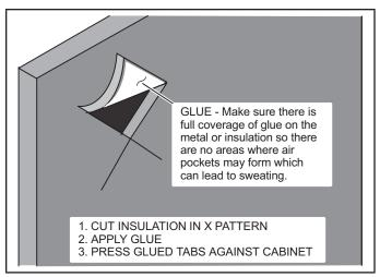
FIGURE 19. Repairing Insulation
