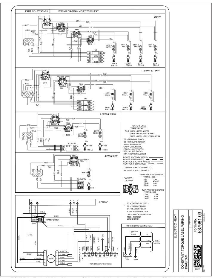
FIGURE 15. Typical Wiring Diagram – CBA25UH Air Handler with Electric Heat – CT (048, 060 models)
