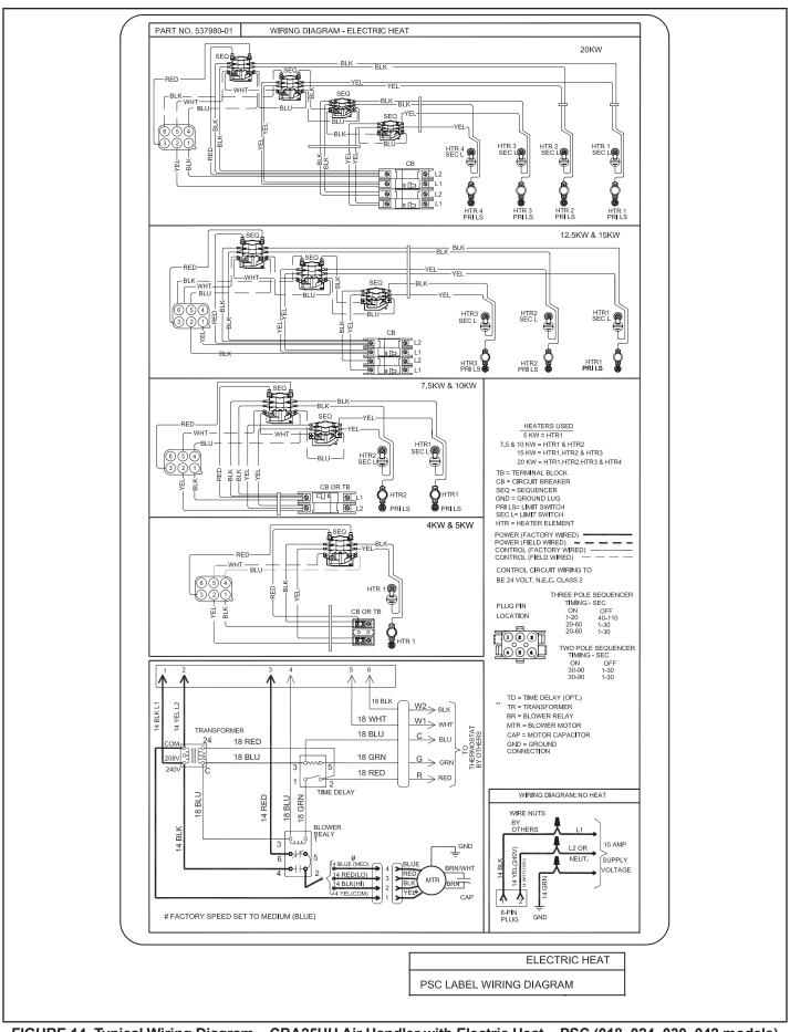
FIGURE 14. Typical Wiring Diagram – CBA25UH Air Handler with Electric Heat – PSC (018, 024, 030, 042 models)
