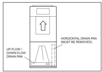
FIGURE 1. Upflow Configuration HORIZONTAL APPLICATIONS
