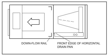
FIGURE 5. Left-Hand Discharge Configuration
