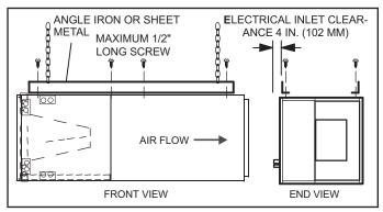
FIGURE 3. Suspending Horizontal Unit
