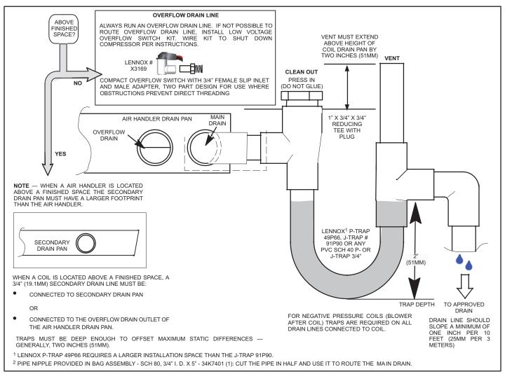
FIGURE 6. Typical Main and Overflow Drain
