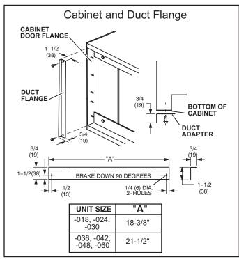
FIGURE 9. Cabinet and Duct Flange
