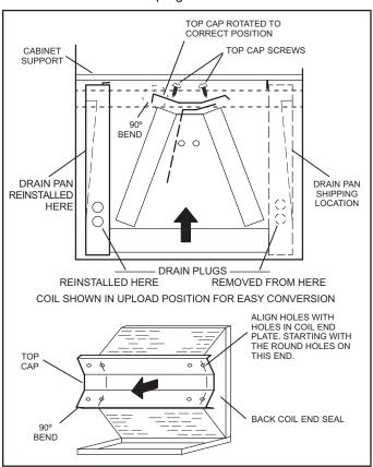
FIGURE 4. Field Modification for Left-Hand Discharge
