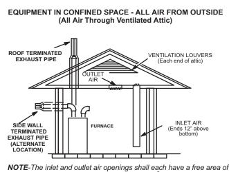
**NOTE**- The infet and outlet air openings shall each have a free area of at least one square inch per 4,000 Btu (645mm<sup>2</sup>per 1.17kW) per hour of the total input rating of all equipment in the enclosure.
