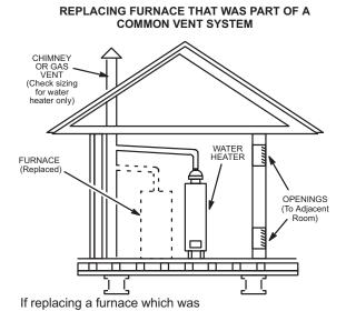
commonly vented with another gas appliance, the size of the existing vent pipe for that gas appliance must be checked. Without the heat of the original furnace flue products, the existing vent pipe is probably oversized for the single water heater or other appliance. The vent should be checked for proper draw with the remaining appliance.
