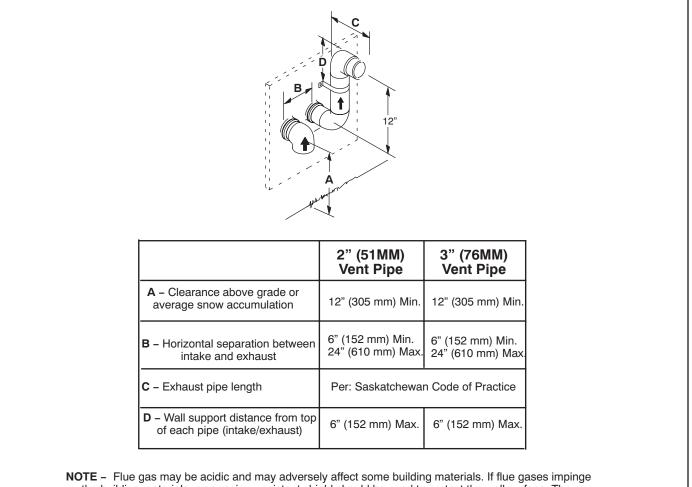
on the building materials, a corrosion-resistant shield should be used to protect the wall surface. The shield should be constructed using wood, sheet metal or other suitable material. All seams, joints, cracks, etc. in affected area, should be sealed using an appropriate sealant.
