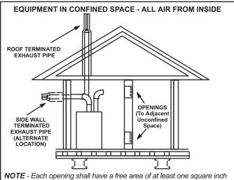
**NOTE** - Each opening shall have a free area of at least one square inch per 1,000 Btu (645mm<sup>2</sup> per .29kW) per hour of the total input rating of all equipment in the enclosure, but not less than 100 square inches (64516mm.<sup>2).</sup>
