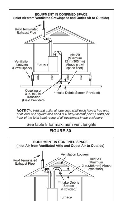
**NOTE**-The inlet and outlet air openings shall each have a free area of at least one square inch per 4,000 Btu (645mm<sup>2</sup>per 1.17kW) per hour of the total input rating of all equipment in the enclosure.
