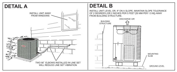
FIGURE 3. Placement and Slab Mounting
