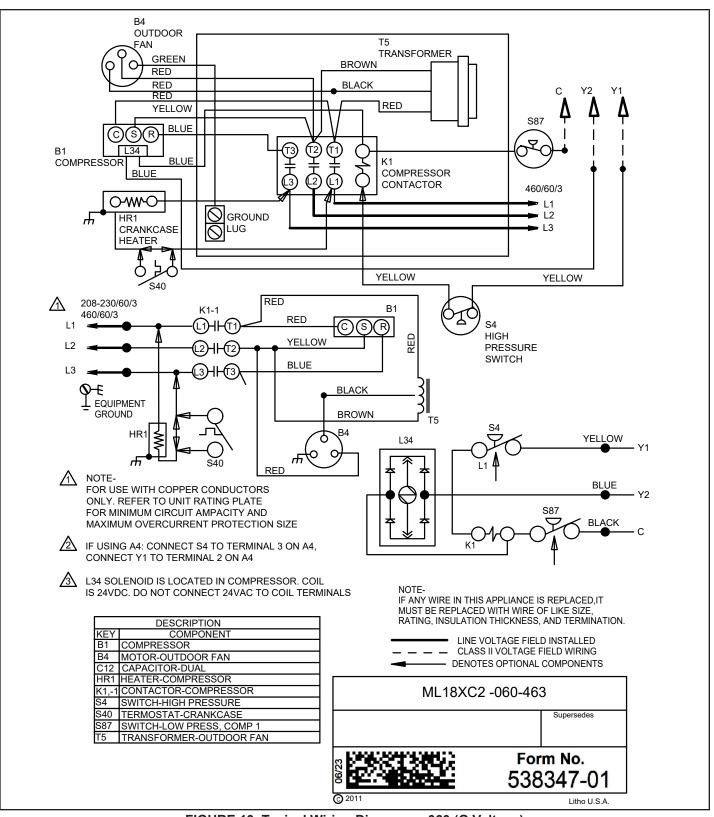
FIGURE 13. Typical Wiring Diagram – -060 (G Voltage)
