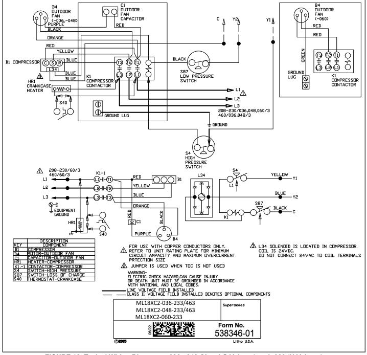
FIGURE 12. Typical Wiring Diagram - -036, -048 (Y and G Voltage) and -060 (U Voltage)
