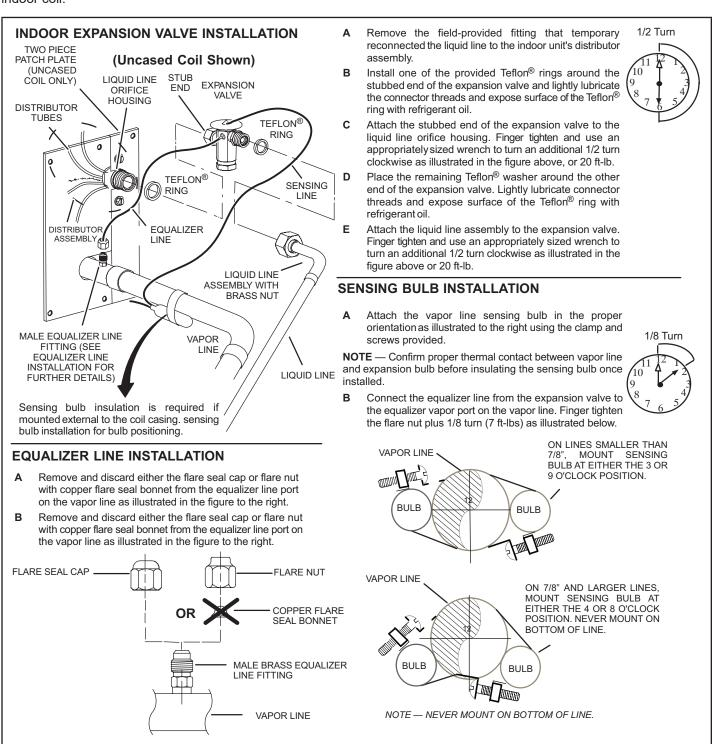
FIGURE 9. Installing Indoor Expansion Valve
