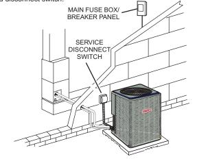
NOTE — Units are approved for use only with copper conductors. Ground unit at disconnect switch or to an earth ground.
