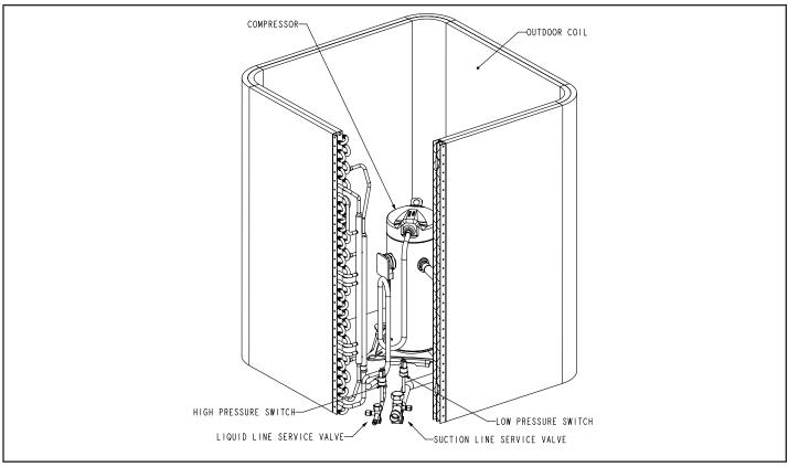
**FIGURE 1. Typical Plumbing Arrangement**
