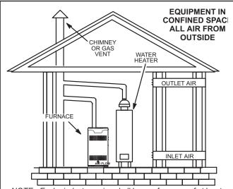
NOTE - Each air duct opening shall have a free area of at least one square inch (645 mm<sup>2</sup>) per 2,000 Btu (.59 kW) per hour of the total input rating of all equipment in the enclosure. If the equipment room is located against an outside wall and the air openings communicate directly with the outdoors, each opening shall have a free area of at least one square inch (645 mm<sup>2</sup>) per 4,000 Btu (1.17 kW) per hour of the total input rating of all other eauinment in the enclosure.
