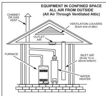
NOTE-The inlet and outlet air openings shall each have a free area of at least one square inch (645 mm<sup>2</sup>) per 4,000 Btu (1.17 kW) per hour of the total input rating of all equipment in the enclosure.
