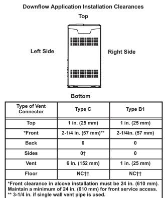
†Left side requires 3 in. if a single wall vent is used on 14 -1/2 in. cabinets, or 2 in. if a single wall vent is used on 17 - 1/2 in. cabinets. ††The furnace may be installed on a combustible wood floor if an optional additive base is installed between the furnace and the combustible floor.
