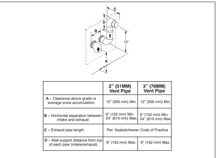
**NOTE** – Flue gas may be acidic and may adversely affect some building materials. If flue gases impinge on the building materials, a corrosion–resistant shield should be used to protect the wall surface. The shield should be constructed using wood, sheet metal or other suitable material. All seams, joints, cracks, etc. in affected area, should be sealed using an appropriate sealant.
